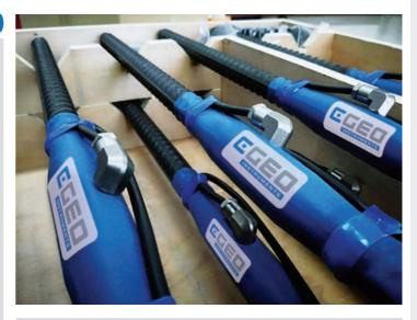
The gauges can be read individually or remotely/automatically as part of a data collection system.
